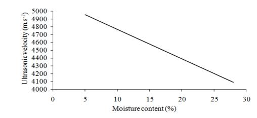
**Figure 1.** Influence of moisture content on ultrasonic pulse velocity in *Eucalyptus grandis* Hill ex Maiden wood. Diagram created from the equation presented in Table 1, with the specific gravity and the base-height ratio (0.5 g.cm<sup>-3</sup> and 3.33, respectively) kept constant.
