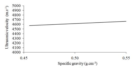
**Figure 2**. Influence of specific gravity on ultrasonic pulse velocity in *Eucalyptus grandis* Hill ex Maiden wood. Diagram created from the equation presented in Table 1, with the moisture content and the base-height ratio (14% and 3.33, respectively) kept constant.
