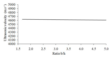
**Figure 3**. Not statistically significant of b/h ratio on the ultrasonic pulse velocity in *Eucalyptus grandis* Hill ex Maiden wood. Diagram created from the equation presented in Table 1, with the moisture content and the specific gravity (14% and 0.5 g.cm<sup>-3</sup>, respectively) kept constant.
