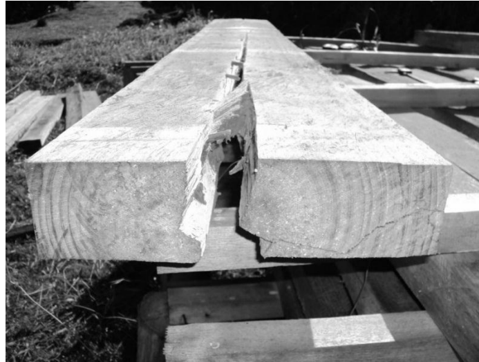
Figure 3. Juvenile wood plank of Eucalyptus grandis presenting end and surface checking.
