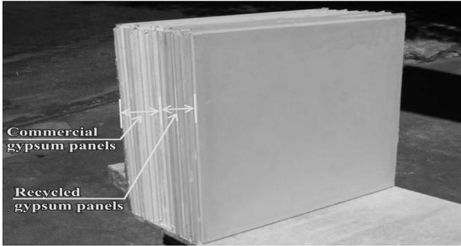
Figure 2. Panels made of recycled and commercial gypsum
