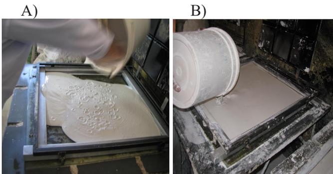
Figure 3. (A) Molding of plaster panels with recycled gypsum (B) Molding of plaster panels with commercial gypsum
