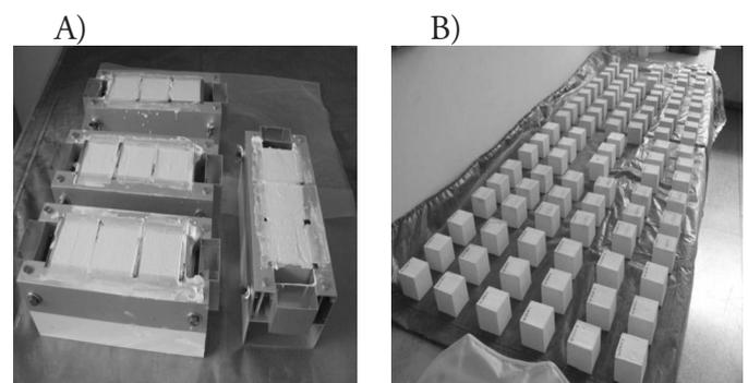
Figure 1. (A) Molding and (B) specimens for compressive strength and water absorption tests
